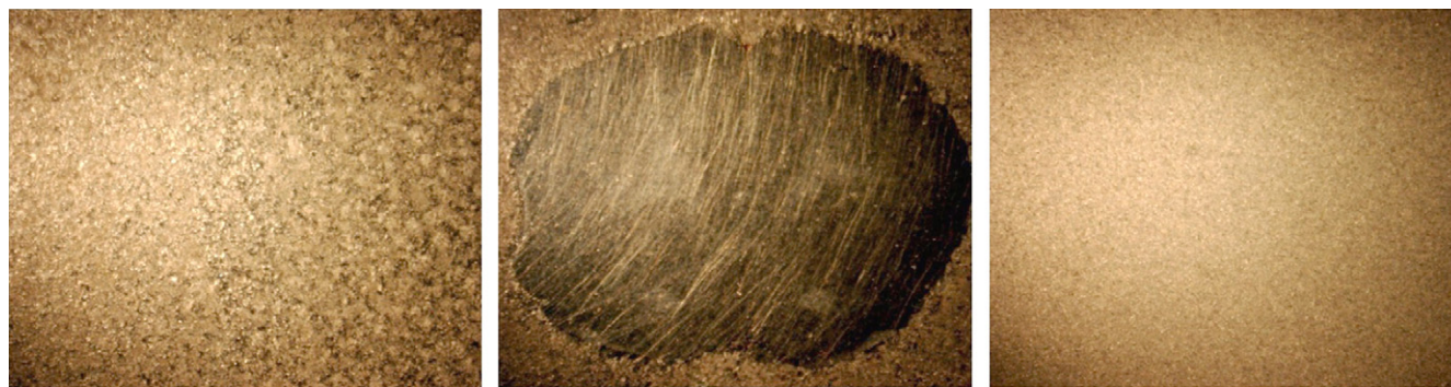
Fig. 1. Surface light microscope pictures of a target plate sprayed with DHB. Left panel: sprayed with TLC sprayer. Middle panel: sprayed with Collision Nebulizer over a tissue section. Note the section was not covered by the matrix. Right panel: sprayed with air brush. Note the homogeneous deposition of matrix over the target surface as compared to the TLC deposition method. Scale bar: 5 mm.
